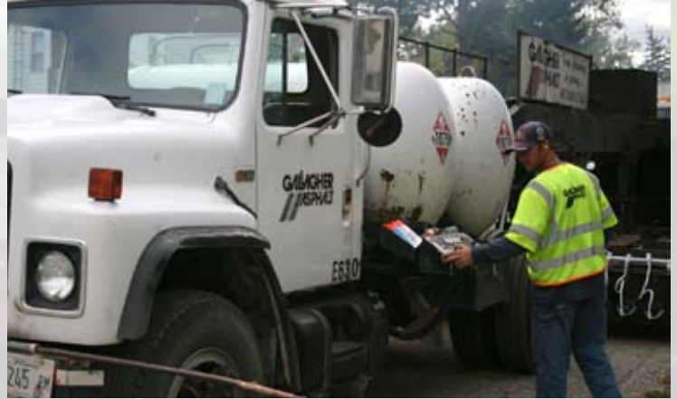
Both vehicles are operated using a computer affixed to the exterior.
